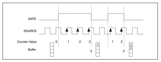
Figure 7-7. Buffered Pulse-Width Measurement
